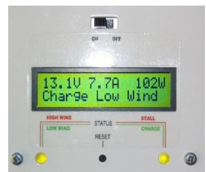
MPC1 Electronic controller with digital display (shown) is included.
