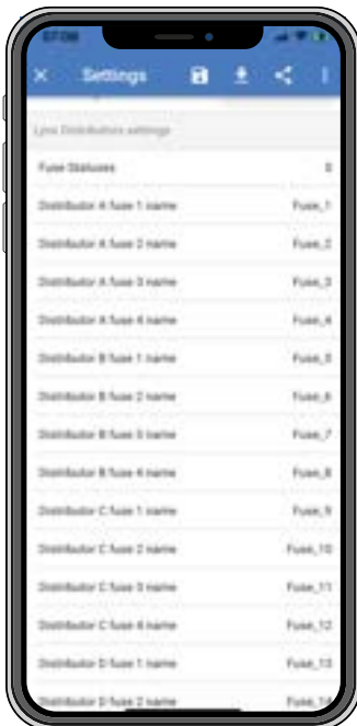
Setting the Lynx Distributor fuse names using VictronConnect
